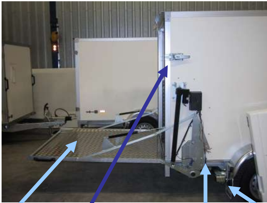
1. load platform 2. draw bolt locking mechanism 3. adjustment bolt 4. support
