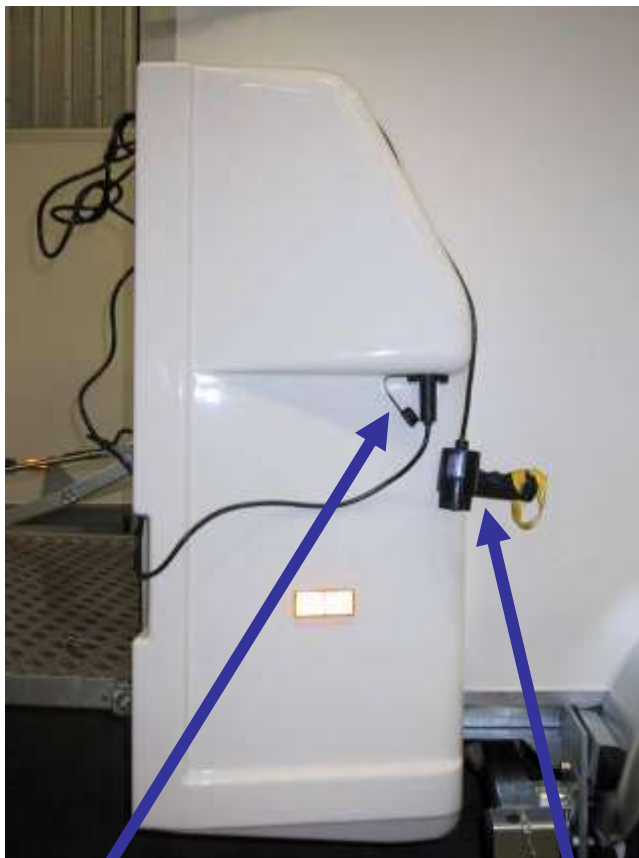
5. connection socket for remote control unit 6. remote control
